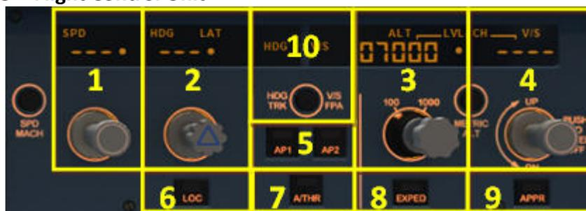
Bild 16: FCU – Flight Control Unit
