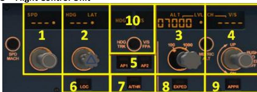
Bild 16: FCU – Flight Control Unit
