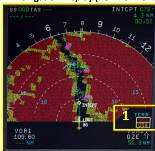
Bild 14: ND – Navigation Display (Takeoff at LOWI 08)
