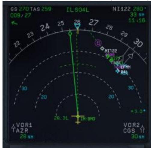
Picture 90: ND flight path after DIR TO and RADIAL IN
