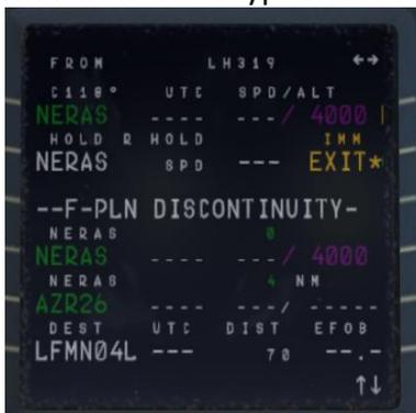
Picture 78: After entering VIA NERAS for new approach
