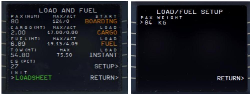
Picture 46: Load/Fuel Menu after INIT LOADSHEET
