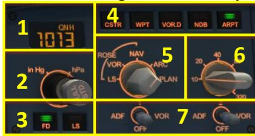
Picture 15: EFIS – Electronic Flight Information System
