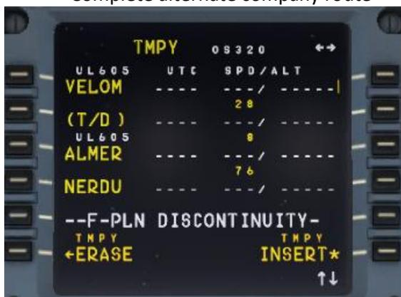
Picture 132: Temporary flight plan after enabling ALTN
