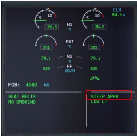
Picture 115: UPPER ECAM – Steep Approach Button = ON
