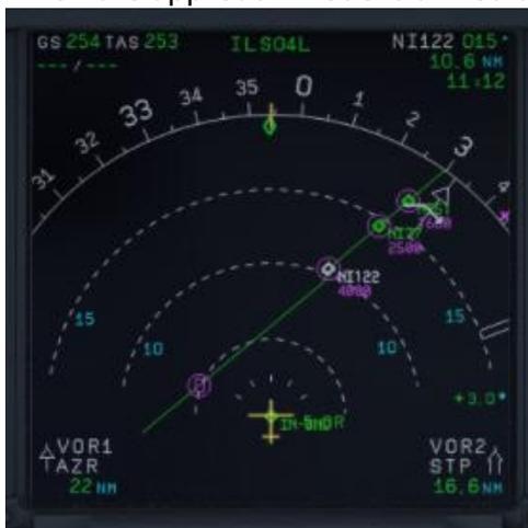
Picture 93: ND flight path after arming APPR mode
