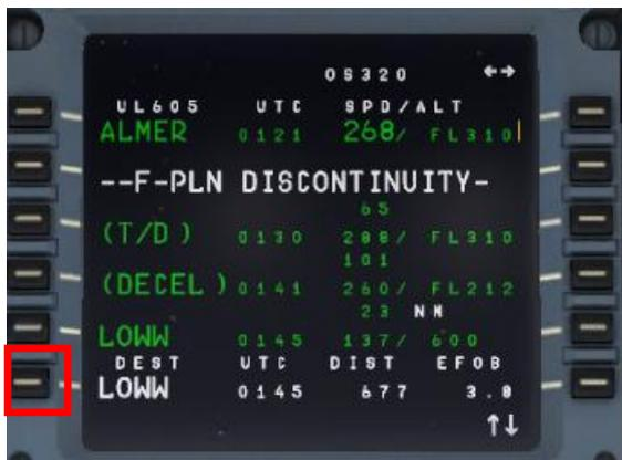
Picture 141: Active flight plan after enabling ALTN
